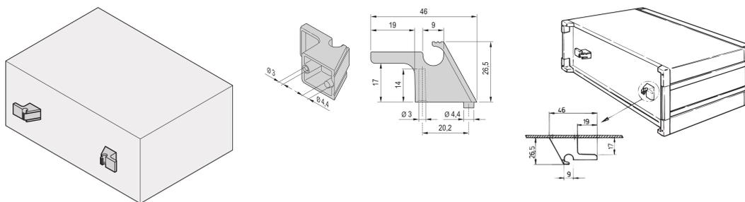
The cable holder enables the fixing of cables. The adapter can be assembled onto a rear panel.
