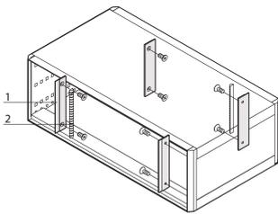
For vertical EMC shielding between front or rear panel and side panel. The bracket can be screwed to the side panel and accepts textile or stainless steel shieldings.
