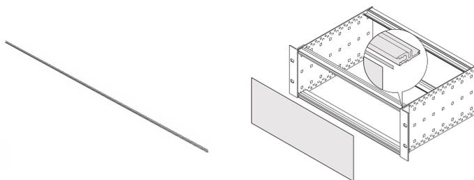
The contact strip clips onto the horizontal rail and makes the contact to front or rear panel.
