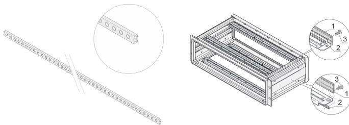
The threaded insert is a metal strip with thread M2.5 and allows the fixing of front panels.
