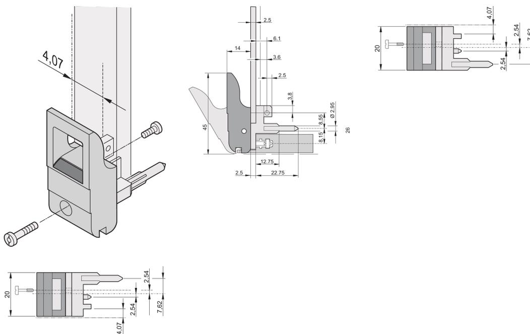
The inserter/extractor handle, type IET in accordance with IEEE 1101.10. Two of these handles can overcome a single lever force of 700 N (per pair).
