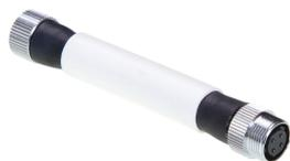
nVent RAYCHEM TraceTek TT-WL-XX-MC is a modular weighted length component with metal connectors, used to provide clear division between areas in a sensing circuit. The weighted length simulates 4.5 m / 15 ft of sensing cable length.
