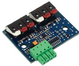
nVent RAYCHEM Elexant 450c plug-in is a sensor module to allow replacement of old controls without stripping insulation and replacing sensors.
