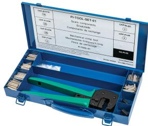
nVent RAYCHEM PI-TOOL-SET-01 is a metal toolbox containing a mechanical crimp tool, crimping dies and the crimps required for the connection of PI heating cables and cold leads in conjunction with the connection/splice kit type CS-150-2.5-PI (cross section up to 2.5 mm<sup>2</sup>).
