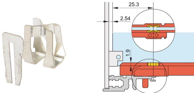
ESD clip ensures conductive contact between PCB and horizontal rail both on the solder side and on the component side.
