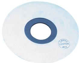
Sealing disks are typically used in vertical pump fill applications, such as columns and shear walls. The sealing disk prevents bedding mortar from entering into the sleeve during installation and grout filling.
