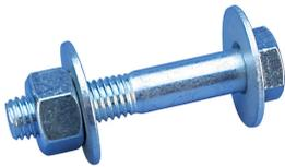
The nVent LENTON Interlok Bolted Form Mount is designed for use with nVent LENTON Interlok Grommet. These kits/bolts are used to secure nVent LENTON Interlok Grout-Fill Coupler variants in repeatable locations in the formwork. Once a Grout-Fill Coupler is placed over a Grommet, the Bolted Form Mount is tightened, which expands the Grommet, thus holding the Grout-Fill Coupler in place.
