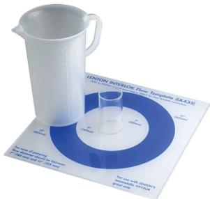
Properly mixed grout is a key to ensuring proper performance of the nVent LENTON Interlok Splicing System. The HY15LM Flow Kit is used to perform a modified slump test exclusively with nVent LENTON Interlok HY15LM Grout.
