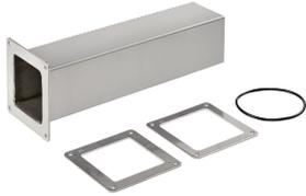
Feed-Through Stainless Steel Telescope Fittings are for adjusting wireway length without cutting or welding. Length is easily adjustable from 1.50 in. to 13.50 in. (343 mm). Connects to other wireway sections and fittings and protects wires and cables in frequently hosed down, very wet or highly corrosive applications.
