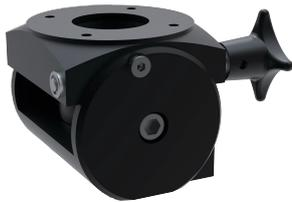
Syspend 281-Max Angle Adapter enables enclosure angle to be adjusted forward or backward up to 30 degrees. Must be used in conjunction with a coupling (not compatible with S2MFC48). Maximum load bearing capacity is 67 lb. (30.4 kg).
