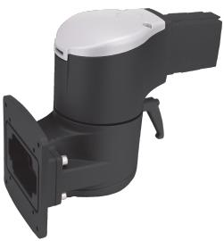
Sysspend 180-Max Horizontal Panel Coupling mounts a horizontal tube to the back of an enclosure or screen using Video Electronics Standards Association (VESA) mounting. The coupling has mounting holes drilled for standard VESA 75 and 100 flange sizes. It enables the enclosure to rotate 300 degrees and can be locked into a given position. The horizontal panel coupling has a safety stop and maintenance-free bearings.
