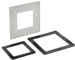
Feed-Through Stainless Steel Reducer Bushings are for reducing to a smaller wireway size. The center hole bushing centers the two wireway sizes relative to each other while the edge hole bushing keeps the top surfaces even. Connects to other wireway sections and fittings and protects wires and cables in frequently hosed down, very wet or highly corrosive applications.
