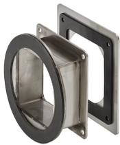
Feed-Through Swivel Nipples are used for adjusting wireway to different angles. Regular type is used between adjacent wireway sections or fittings while the box entry type is used when entering an enclosure. Connects to other wireway sections and fittings and protects wires and cables in frequently hosed down, very wet or highly corrosive applications.
