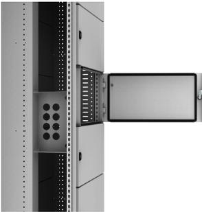
This galvanized cable entry box, MSCE, covers a partial depth of the enclosure. It has been tested according to IEC 61439, complies with form 4, and is available off the shelf. The box separates cable terminations from each functional unit and makes the terminations inaccessible from the cabling section, which in turn reduces potential health and safety hazards. Labour time to be spent is short as the holes for cable entry are pre-machined.
