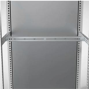
This profile, APK, can be continuously adjusted both in height and depth in an enclosure. Cage nuts, that may be adjusted in width, can be fitted onto the profile to allow for flexible mounting of various components.
