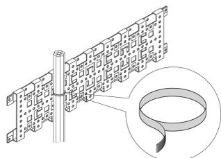
Velcro® Strip is one of the simplest cable bundling solutions. nVent SCHROFF Velcro® strip allows up to 43 mm diameter of wires.
