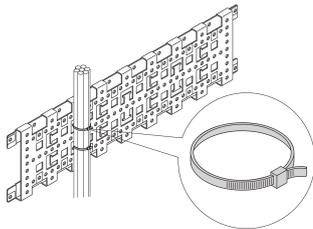
Assembling materials kit for cable routing.
