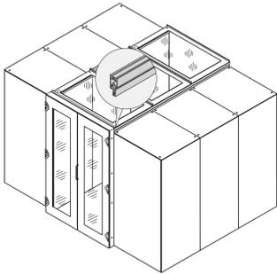
Profile that allows the easy fixing of aisle top covers.
