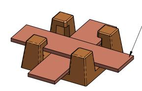
2: Insert one or two coper tape 25x3 mm in cross configuration (like the example) or in T configuration
