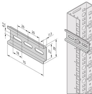
DIN rail for thermostat or hygostat clamping.
