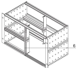
The 2 HP wide front panel covers an open slot. The U-profile front panel can be combined with a textile EMC gasket. It be fixed with screws and washers. Due to the 2 HP width no sleeves can be used.
