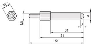
This coding peg / pin enable a safe connection between the floating connectors used for the SNCF subracks. The Pins can be assembled into the rear frame.
