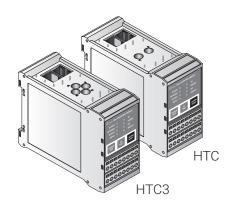
The NGC-40 uses a single controller module per heat-tracing circuit for maximum reliability. The NGC-40 control system can be powered between 100 to 240 Vac, while mechanical contactors (EMRs) or solid-state relays (SSRs) allow circuit switching up to 60 A at 600 Vac.
