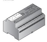
The NGC-40 works with the MONI-RMM2 module. Each RMM2 module installed in the field can accept up to 8 RTDs. 16 RMM2 Modules can be daisy chained together via RS-485 for a total of 128 temperature inputs. Since multiple RMM2s can be networked over a single cable to the NGC-40, the cost of RTD field wiring will be significantly reduced.
