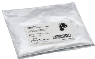
The nVent LENTON HYA15LM Grout Additive, Hot Temperature is designed to be used in conjunction with nVent LENTON Interlok grout-fill couplers and nVent LENTON Interlok HY15LM Grout. The additive is used to increase working time of the grout during hot temperature applications which allows for a longer time window to place the grout into the Interlok couplers. This proprietary grout additive increases the maximum working temperature of HY15LM grout from 100 °F (38 °C) to 122 °F (50 °C).
