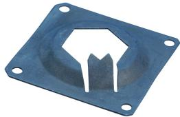
The HFF nailing plate is sold separately from the A12 couplers. The plates easily attach to the couplers by orienting the hexagon opening in the plate to the coupler and then rotating the plate 15 degrees.
