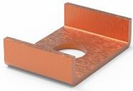
This busbar holder, MSBH, has been tested according to IEC 61439 and is available off the shelf. It is easy to mount and connects two bars with a thickness of 10 mm, to create a proper contact for an attached electrical cable.
