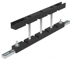
This busbar support, ECBS, is available for one or two bars up to 80 x 5 mm or one bar up to 80 x 10 mm. The support can be mounted both horizontally and vertically. It is available off the shelf and tested according to IEC 61439.
