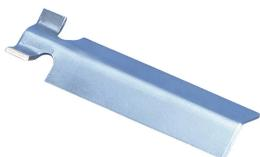
nVent LENTON Speed Sleeve Transition Adaptors allow the nVent LENTON Speed Sleeve to be used as a transition splice. The transition adaptors are simply placed inside the sleeve underneath the straps of the smaller bar end.
