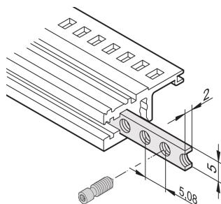
The threaded insert is a metal strip with thread M2.5 and allows the fixing of front panels.
