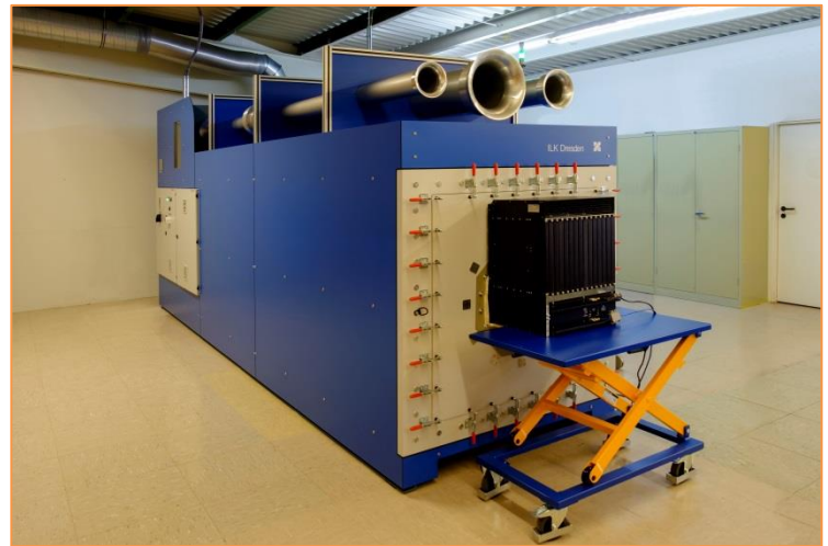
Figure 1 Air performance test rig_1
