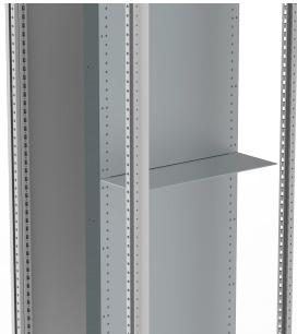
This steel zinc plated separation plate, MSISM, is available off the shelf and pre-sized. The plate should be used when subsections need to be segregated. It is placed between a mounting plate and a front panel that is placed inside the enclosure. No screws are needed, which makes mounting easy. The fix section can then comply to up to form 4 segregation according to IEC 61439.
