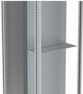
This polycarbonate horizontal separation plate, MSIS, is available off the shelf and pre-sized. The plate should be used when subsections need to be segregated. It is placed between a mounting plate and a front panel that is placed inside the enclosure. No screws are needed, which makes mounting easy. The fix section can then comply to up to form 4 segregation according to IEC 61439.
