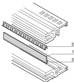
The contact strip makes contact between horizontal rails. If two horizontal rails are mounted one above the other, the seals plus a metal strip enable EMC shielding.
