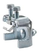
This code-compliant Structural Attachment is part of the nVent CADDY line of innovative rigid bracing system, designed to provide superior performance and meet the highest seismic load requirements. Its innovative design allows quick and easy installation onto both top or bottom flange of a wide range of steel I-Beams. Its snap-off bolts make inspection of seismic sway braces simple.
