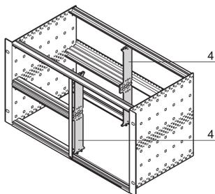
The support is bolted into the grid holes of the horizontal rails and allows a split of a 6 U subrack in 2 x 3 U parts.
