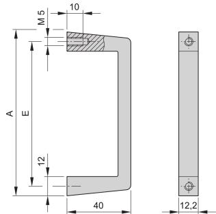
The handle can be assembled to a subrack or 19" front panel. Available with clear or black anodized surface. Handles will be bolted from the rear side.
