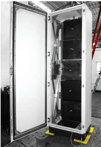
Figure 8. MCS20088R5 With seismic kit, seismic plinth and loaded mounting plate.
