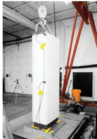
Figure 9. MCS20088R5 With seismic kit and seismic plinth
