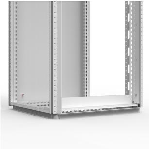
The mild steel modular system frame for floor standing enclosures, MSMSF, has two mounting levels. The first is for fixing front panels and the second for mounting equipment. The frame can be equipped before mounting in the enclosure and allows for the use of both modular and non-modular components.
