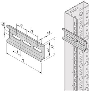
DIN rail for thermostat or hygostat clamping.
