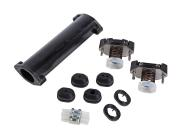
nVent RAYCHEM CS -150-UNI-PI is a universal underinsulation cold applied connection kit for polymer insulated (PI) heating cables, for splicing and connection of PI heating cables to cold leads (max 32A) or 3-core flexible power cableS (max 25A) using screw terminals. Approved for use in hazardous areas.
