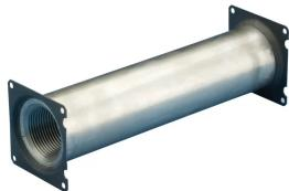
Used in segmental pour applications. The addition of two form saving plates allows the coupler to be used in keyway applications where the coupler is attached to formwork at both ends. Permanent form saving plates allow easy attachment to the forms, eliminating costly damage to the forms.
