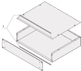
The EMC shielding kit and the cover plates increase the shielding of the chassis from approx. 30 dB(A) to approx. 60 dB(A). A test report can be downloaded.
