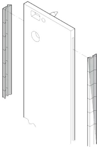
The stainless steel EMC gaskets are inserted into the lateral slots of the shieldable front panels (2 pieces per front panel).
