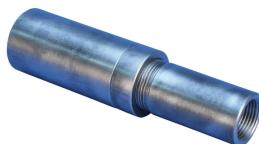
The P24 family of position couplers is designed for use on ASTM A615 grade 100 (700 MPa) reinforcing steel. The performance of the spliced connection is designed to meet the bars' specified ultimate tensile strength of 115 ksi (792 MPa).
