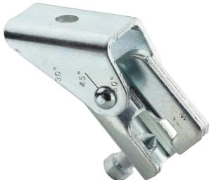
This code-compliant Structural Attachment is part of the nVent CADDY line of innovative rigid bracing system, designed to provide superior performance and meet the highest seismic load requirements. Its versatile design allows quick and easy installation directly to concrete, wood, bar joist or I-beam adapters and is compatible with 1" through 2" brace pipes. Its snap-off bolt makes inspection of seismic sway braces simple.
