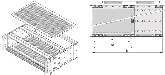
A cover plate is used for electromagnetic shielding or as mechanical protection.
